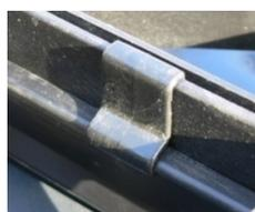
Passing the cord through this beam cleat is made easier by using masking tape wound tightly over the end of the support cord. Tie a knot in the rope at each end of the beam once you've inserted the beam cleats. Grids are placed onto the beam lengthways (i.e. the side of the grid that is 59cm long).
